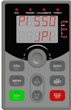
Figure 3-1: Operation panel display
